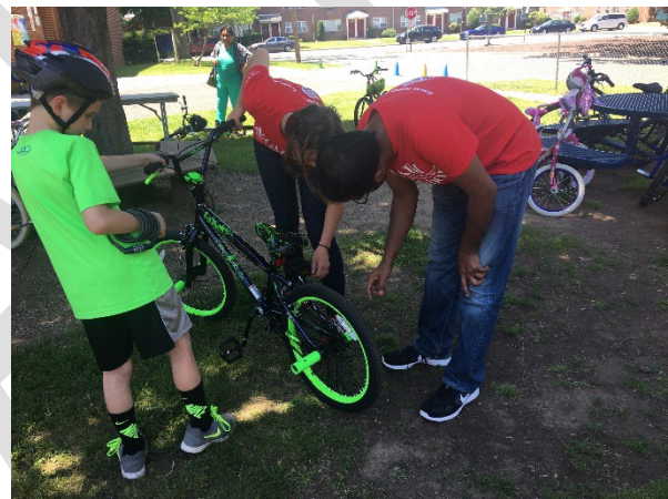
Ambassadors assist a young rider with an 'ABC quick check', checking tire pressure, brakes, and crank set.
