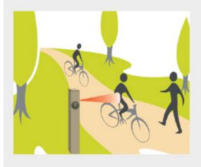
The **PYRO** sensor uses a combination of passive infrared pyroelectric <u>technology</u> and a high precision lens to detect a change in the detected temperature when a person passes in the range of the sensor. Thanks to its extremely high sensitivity, the sensor can detect two different people with only a small gap between them. The sensor is self-calibrating for simple installation.
