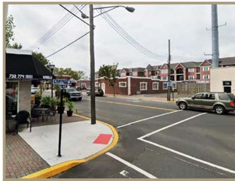
Figure 21. Diagonally aligned curb ramp on Main Street at McCabe Avenue.
