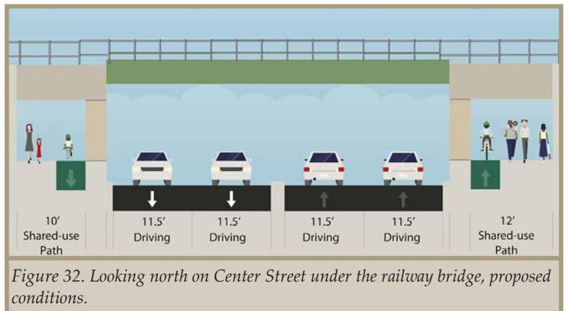
Figure 32. Looking north on Center Street under the railway bridge, proposed conditions.
