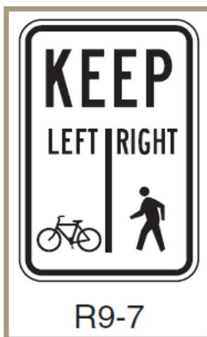
Figure 26. Shared-use path restriction sign (Photo Credit: MUTCD)
