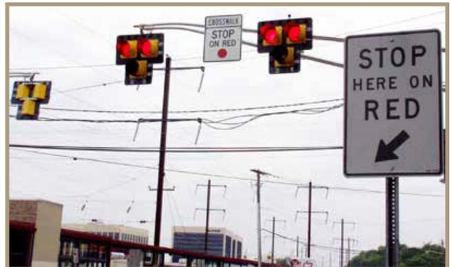
Figure 73. Pedestrian Hybrid Beacon near Metropark Train Station, NJ. (Photo Credits: NJDOT)
