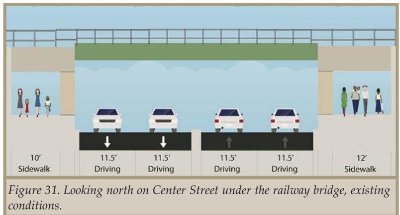
Figure 31. Looking north on Center Street under the railway bridge, existing conditions.
