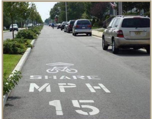
Figure 54. Pavement markings for a bicycle boulevard in Ocean City, New Jersey.
