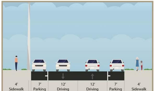
Figure 47. Looking east on Second Avenue in front of the St. Anne’s Convent, existing conditions.
