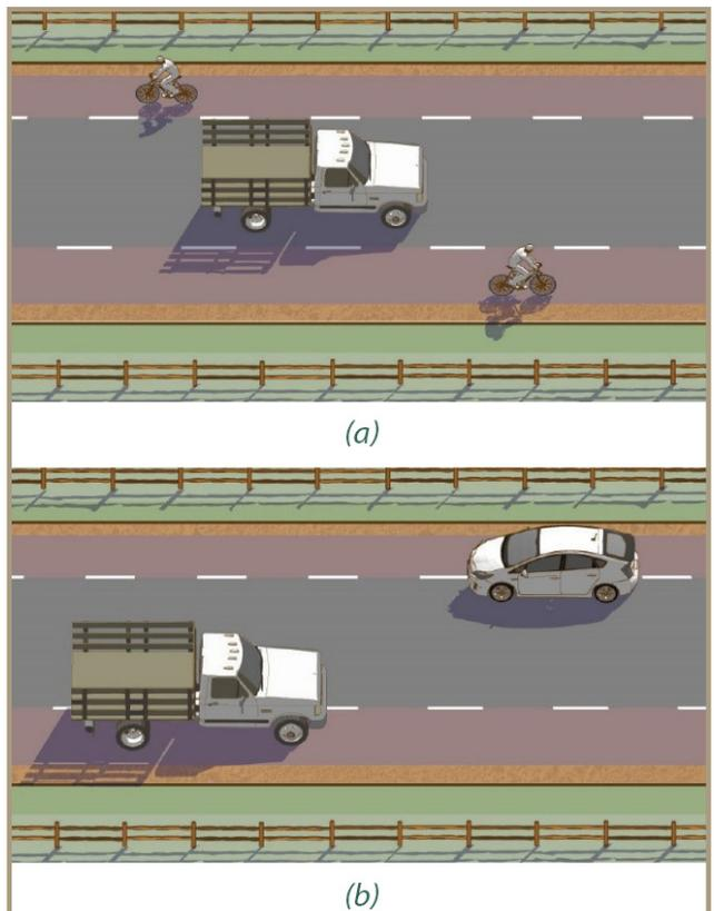
Figure 48. An advisory shoulder with: a) A motorist traveling in the center two-way lane when passing a bicyclist, and b) A motorist using the advisory shoulder to pass an oncoming vehicle when bicyclists are not present.
