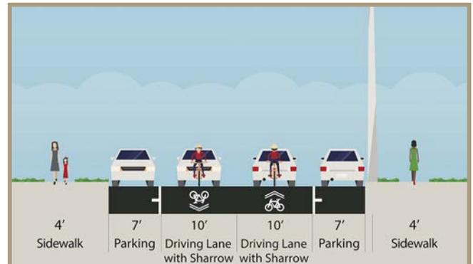
Figure 68. Looking east on Fourth Avenue between Maple Street and Brookside Place, proposed conditions.
