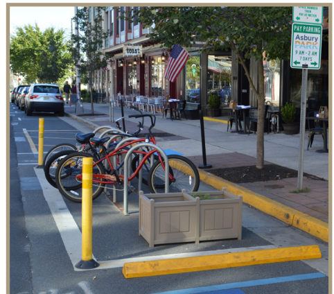
Figure 23. Yellow plastic bollard, parking stop, plastic planter, bike parking. Asbury Park, New Jersey.
