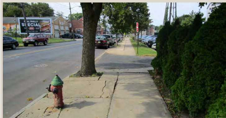
Figure 71. Shrubbery blocking driver's visibility of sidewalk.
