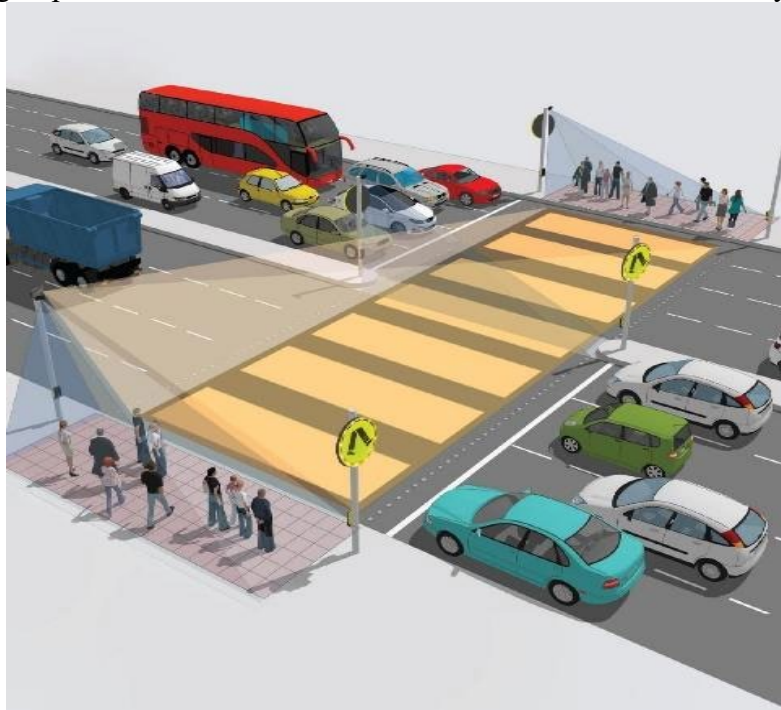
Figure 18. Pedestrian detection system scheme (HI-VIS, 2022)
