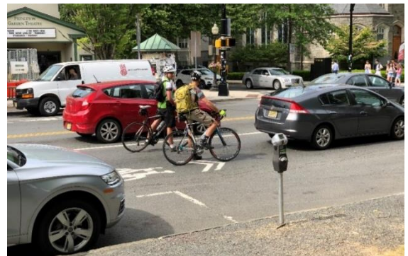
Example of bicyclists on road with shared lane markings in Princeton, NJ
