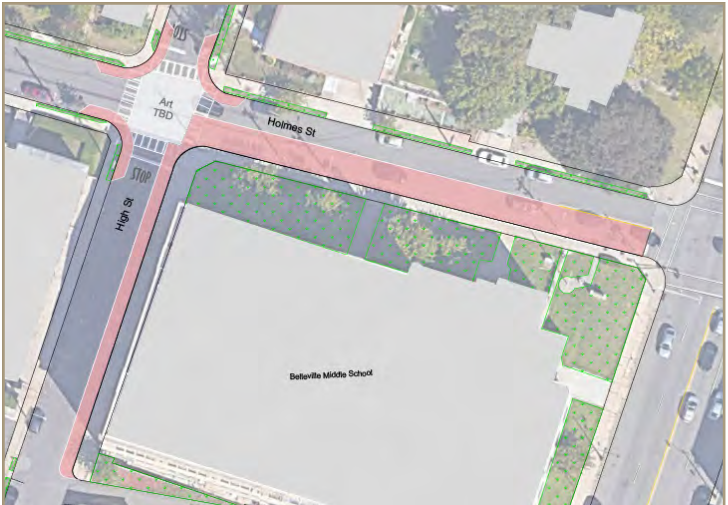
Figure 22. Alternative B, expanded sidewalks at the intersection of Holmes Street and High Street.
