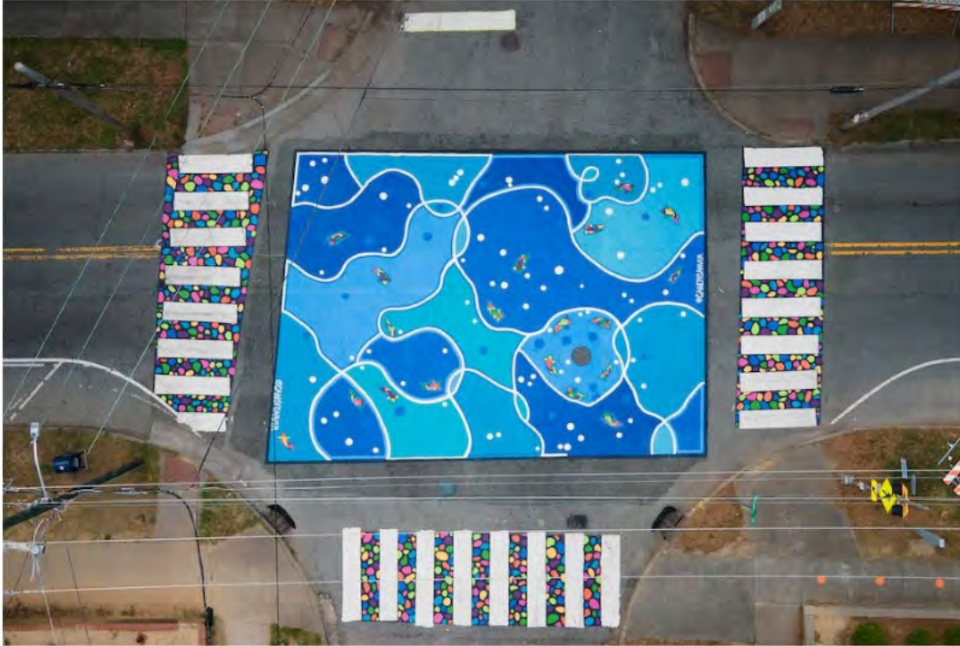
An intersection near an elementary school in Durham, N.C. Since asphalt art was installed last May, potentially dangerous collisions between drivers and pedestrians dipped by 30 percent. (Bloomberg Philanthropies)
