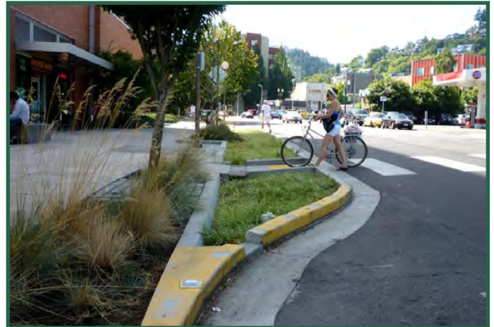
Figure 8. Green infrastructure used to narrow the roadway and provide a shorter crossing distance for pedestrians.
