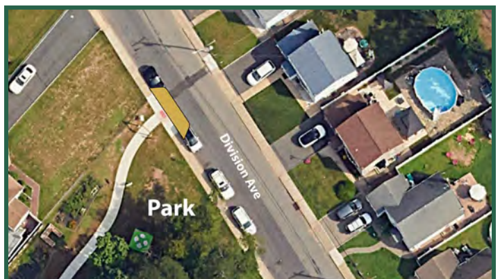
Figure 47. Curb extension in front of pocket park.
