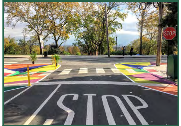
Figure 12. Painted curb extensions in Jersey City. Photo by Street Plans.
