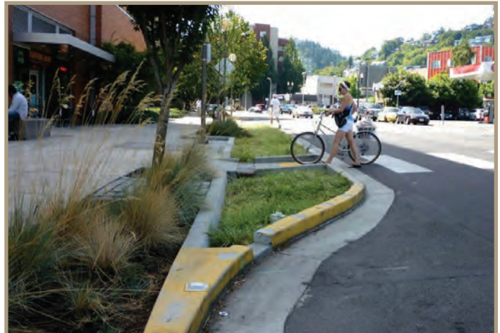
Figure 5. Green infrastructure used to narrow the roadway and provide a shorter crossing distance for pedestrians.
