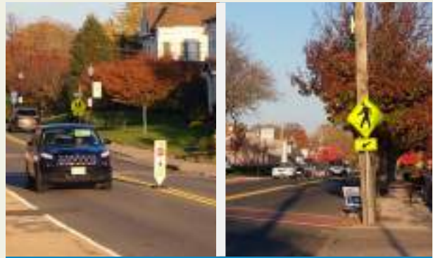
Examples of in-road "Stop for Pedestrian" (left) and pedestrian crossing signage already used in Fair Haven to enhance pedestrian crossings
