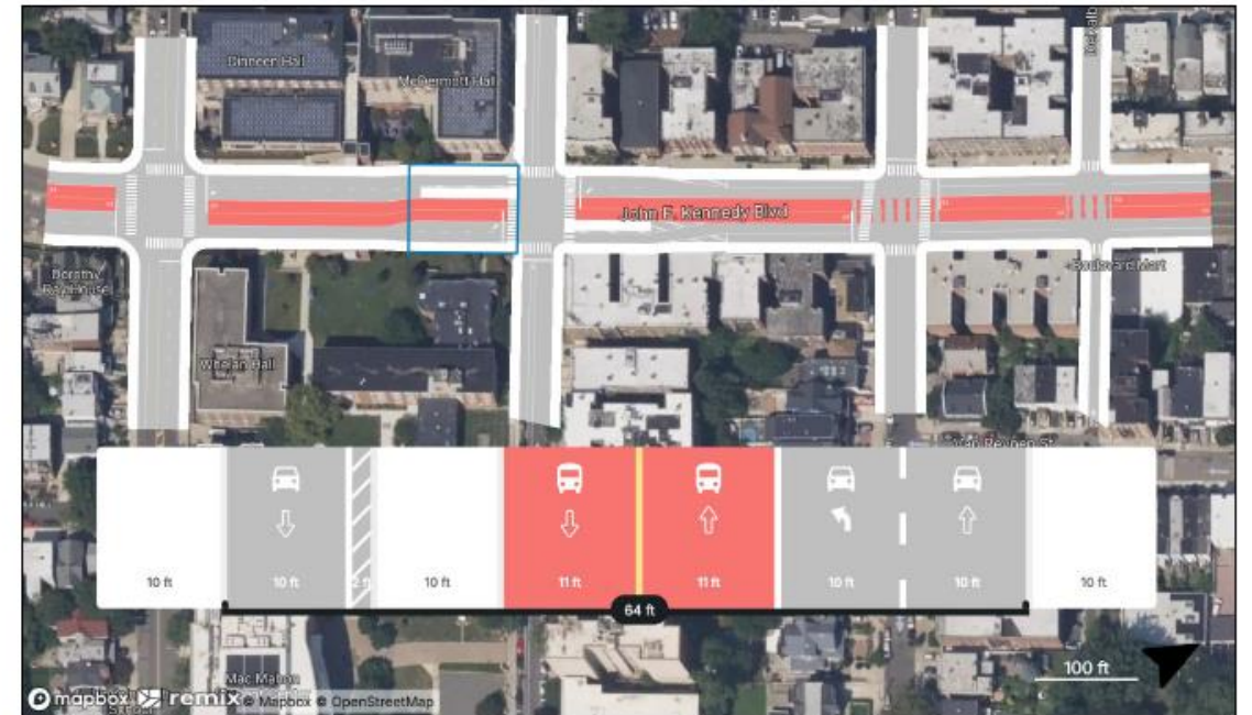
Figure 7 Creative design solutions could improve bus speeds while mitigating traffic impacts (source: Nelson\Nygaard)
