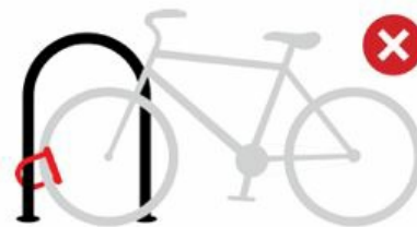
U-Lock secures front wheel only, leaving rest of bicycle vulnerable to theft.
