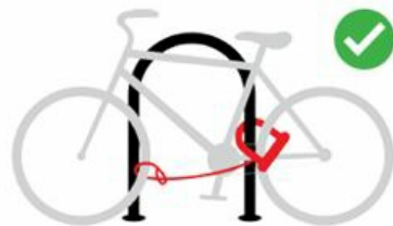
U-Lock secures rear wheel and frame, with additional cable to secure front wheel.
