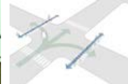
Dedicated Greenway Phases or a Leading Pedestrian Interval (LPI) Can dedicate a signal phase or a portion of a signal phase to greenway travelers only
