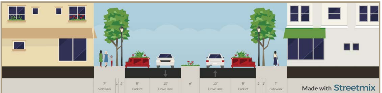
Figure 45. Current parking spaces could be used for parklets with restaurant seating areas, protected bus shelters, and/or curb extensions that shorten long crosswalks and provide space for pedestrian amenities.
