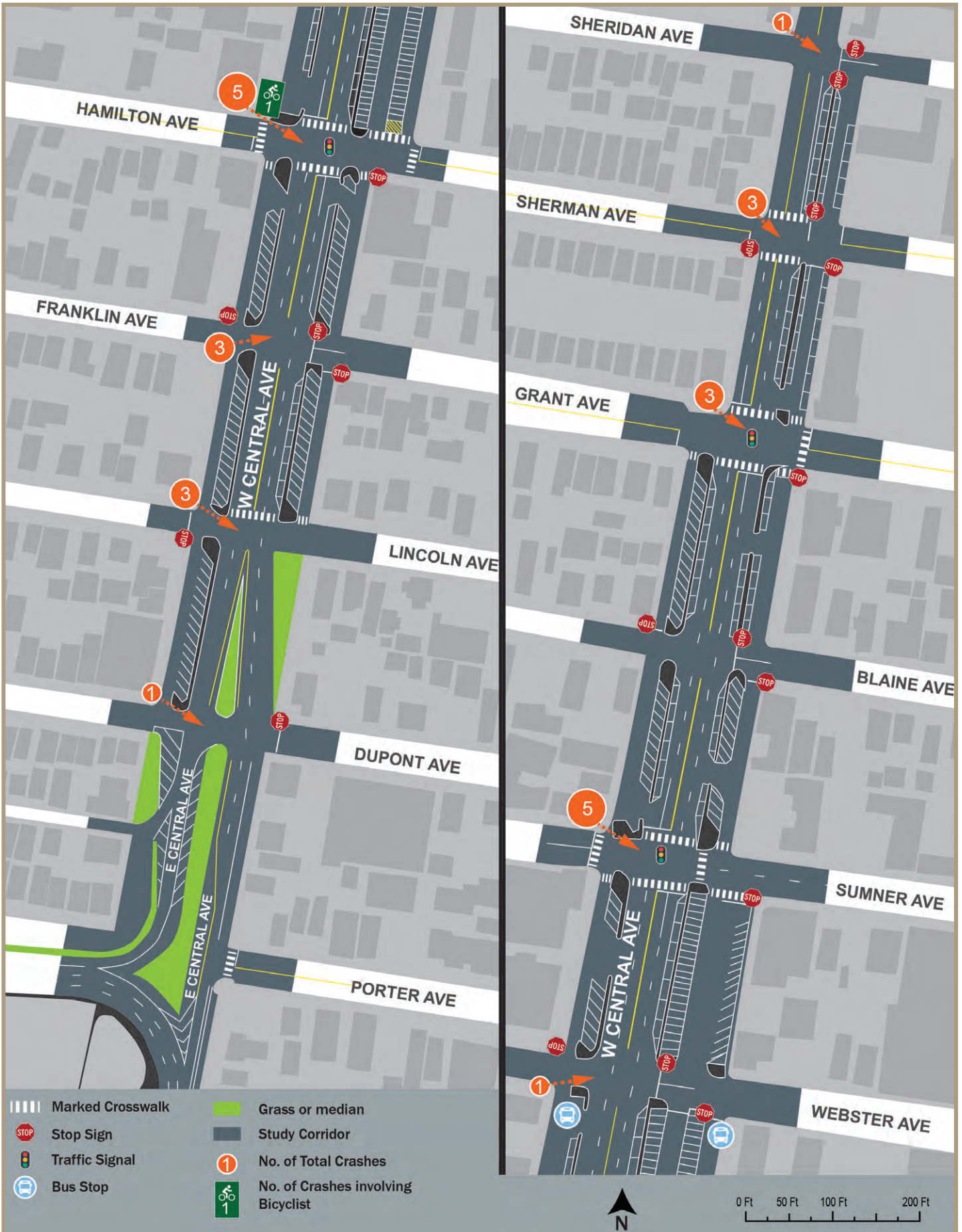
Figure 9. Central Avenue Corridor Map. The number of crashes is shown to the left of the corridor but they represent crashes at the intersection.
