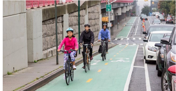
Figure 4: A two-way parking-protected bike lane in New York City, NY (New York City DOT, 2022)
